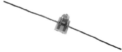
Fig. 4. Self-made dipole antenna that has been used for the measurements
